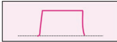
Fig: 8.2: Square flow wave pattern (inspiration)
